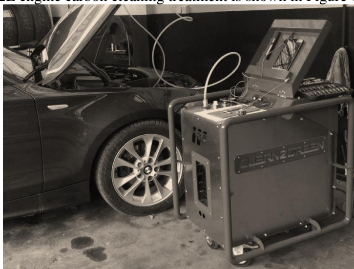
Figure 1. H2E engine carbon cleaning treatment
