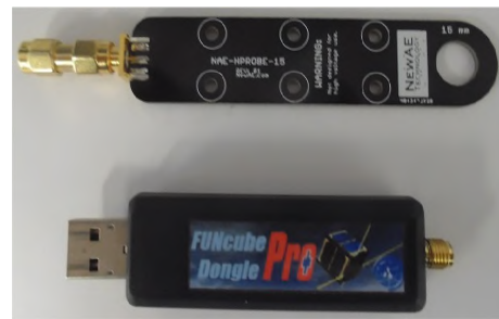
(b) H-field Probe and SDR dongle
