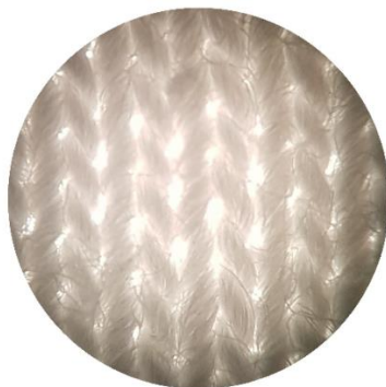
Figure 3.2 Weft Knitted Fabric (Durban University of Technology: 2017).
