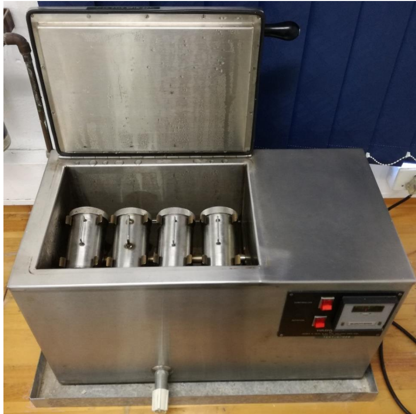
Figure 3.8 James H Heal Washwheel (Durban University of Technology: 2017).
