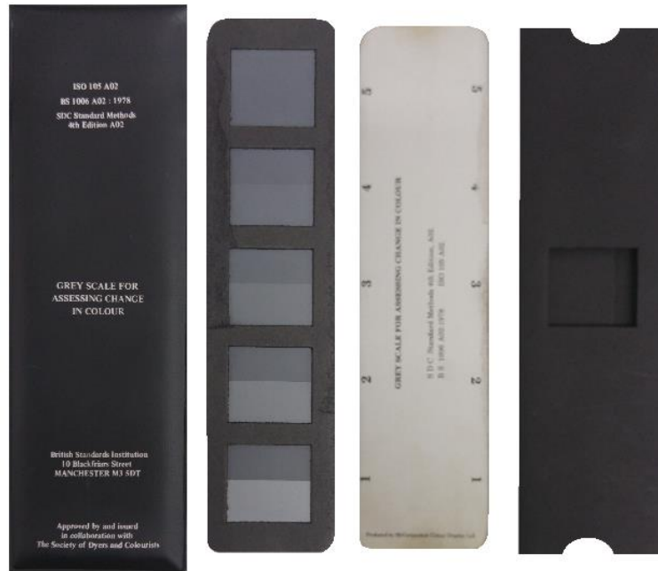
Figure 3.12 SDC Grey Scale for Assessment of Change in Colour (Durban University of Technology: 2017).
