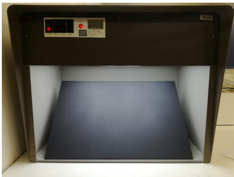
Figure 3.10 Instrumental Colour Systems Ltd Multi-light Box, using D65 Illuminant (Durban University of Technology: 2017).
