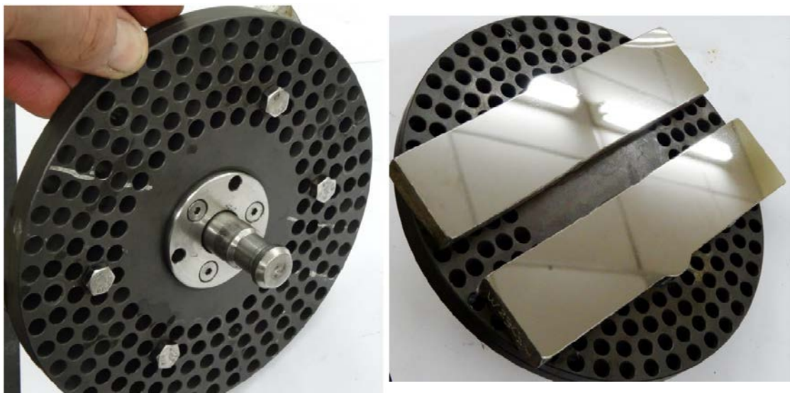
Figure 3-5: An example of how the large macro samples were secured to the universal polishing head (L/H side) and the final polished macro samples (R/H side).
