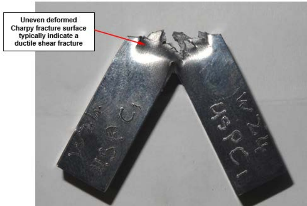
Side view of one of the parent pipe material Charpy Impact samples tested
