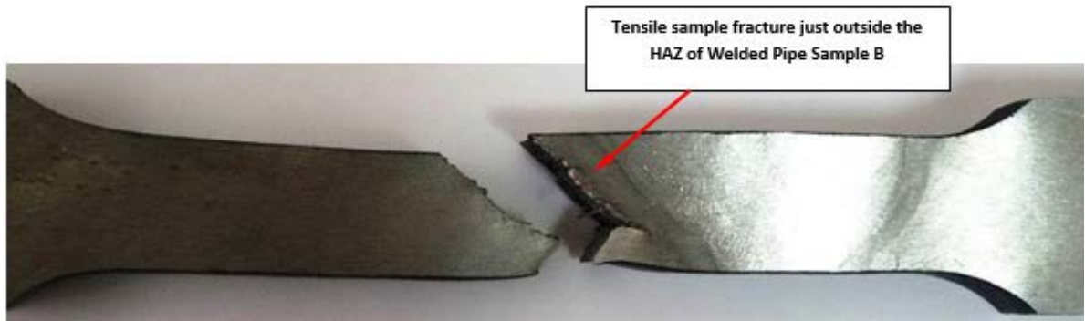
Figure 3-40: The side view of the only HAZ Tensile sample that fracture along the HAZ interface, where high levels of planar graphitization were evident.
