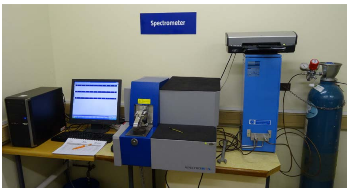
Figure 3-1: The SpectromaxX Spark spectrometer used to determine the bulk chemical composition of the service exposed steam pipe samples.
