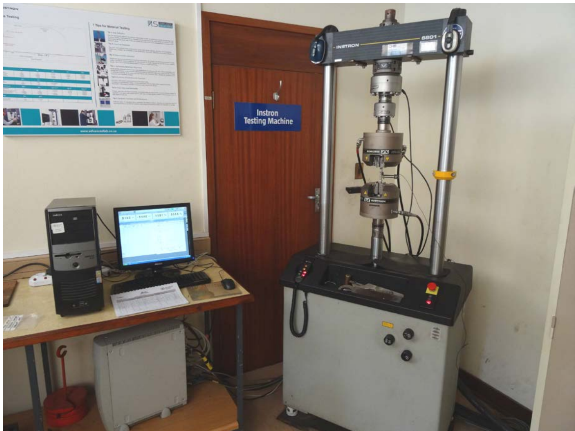
Figure 3-27: The Instron 8801 servo-hydraulic test platform used to perform the room temperature tensile testing of the tensile samples removed from the different service exposed steam pipe regions.
