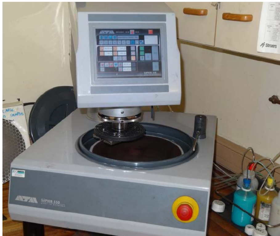
Figure 3-4: The ATM Saphir 550 semi-automatic polishing machine used to fine ground and polish the large macro samples and smaller micro samples.
