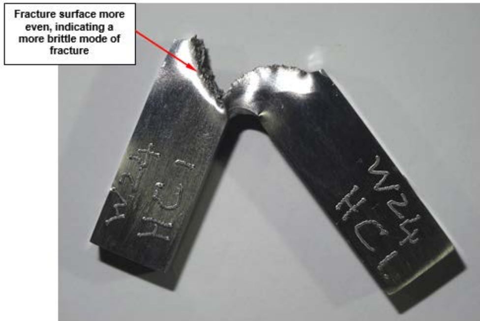
Side view of one of the HAZ material Charpy impact samples tested
