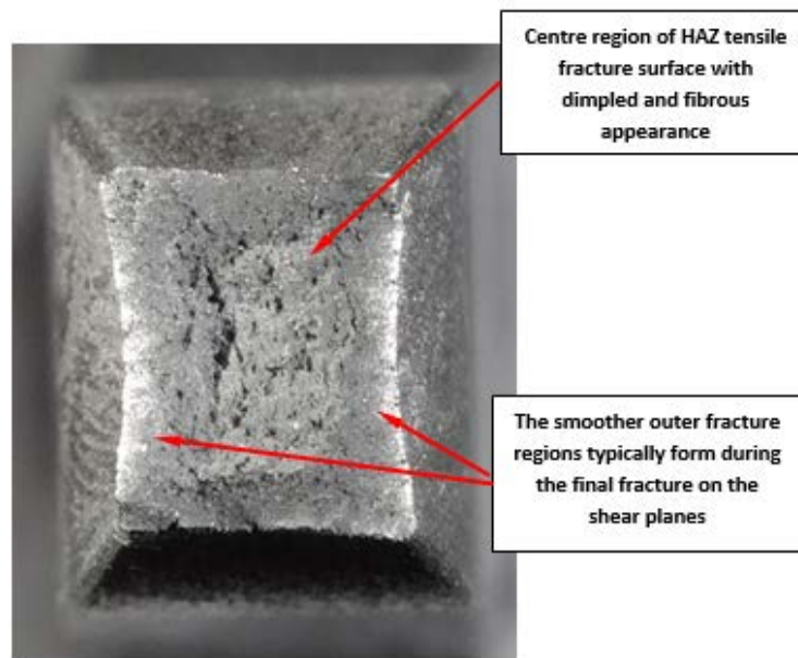
Figure 3-34: Close up view of one of the HAZ tensile sample's necked fracture surface with a dimpled and fibrous appearance, typical of a ductile overload fracture.
