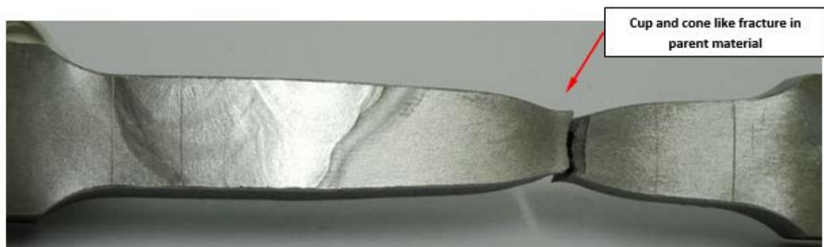
Figure 3-33: A typical example of how the majority of the tensile taken from just outside the HAZ fractured in the parent steam pipe material.
