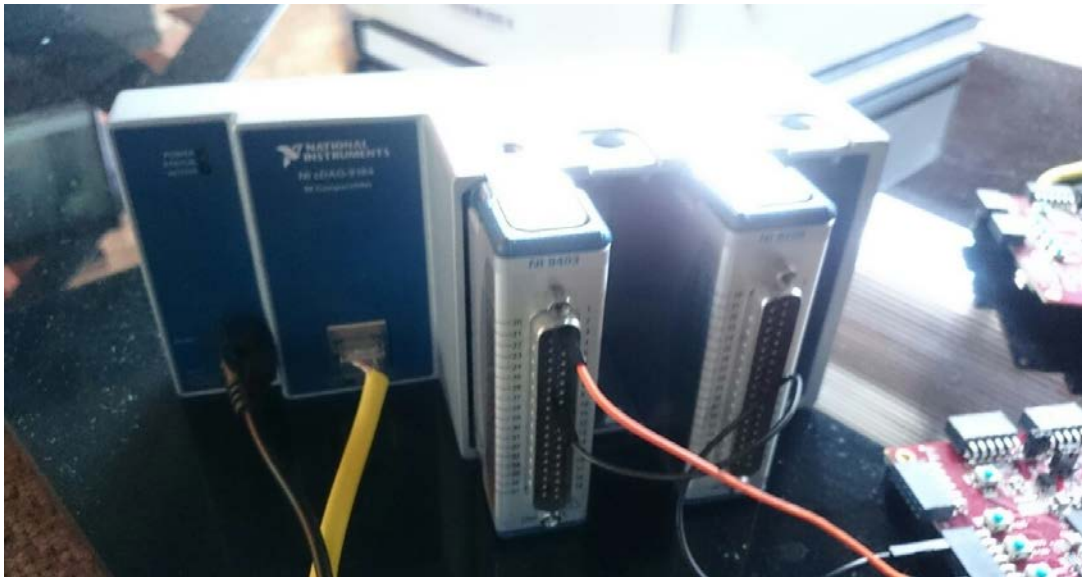
Figure 27 - National Instrument's Compact DAQ used for error counting
