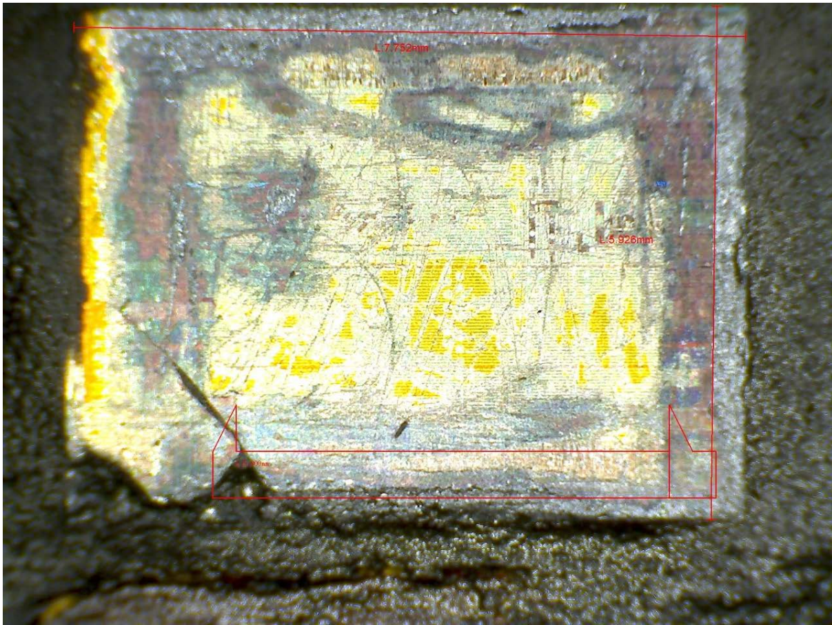
Figure 43 - Decapsulated device to obtain the die area
