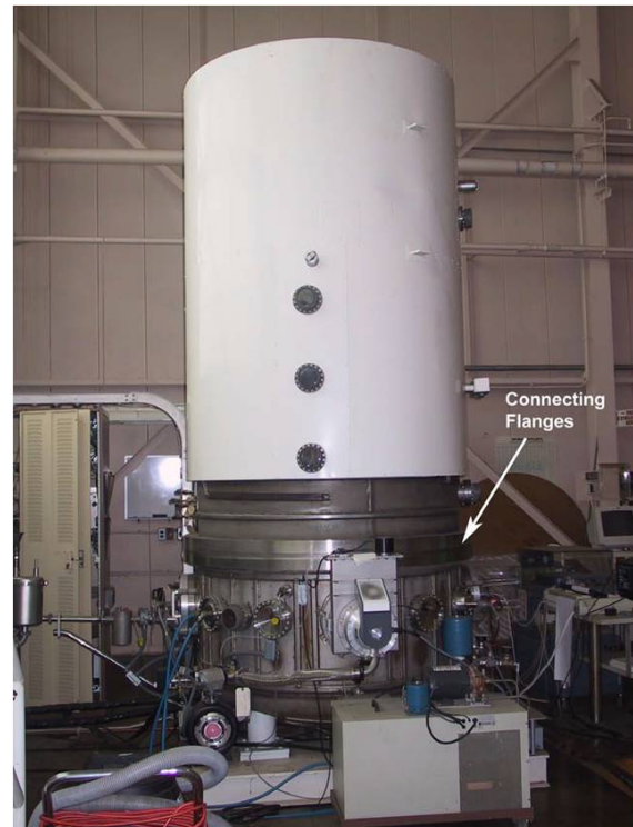
Figure 3: VF-13 test chamber used for pressure rise experiments.
