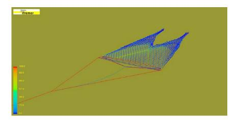
Figure 17. DynamiT simulation of T-Line net.
