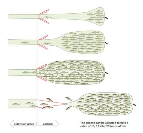
Figure 3. Working principle of the detaching codend.
