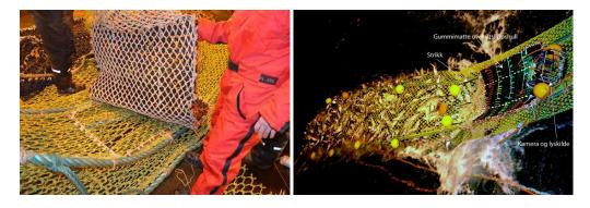
Figure 9. Catch control device based on a rubber mat and a fish lock (Source: CRISP)
