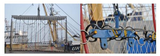
Figure 16. T-Line elements on a SumWing (left) and detailed (right).
