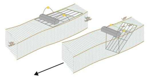
Figure 7. Active catch release system: Motorized gate that opens up on a signal from an operator.
