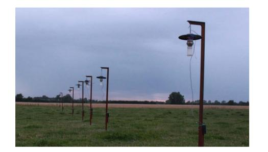
10 light traps were placed on a line in a symmetric pattern with less distance towards the middle.
