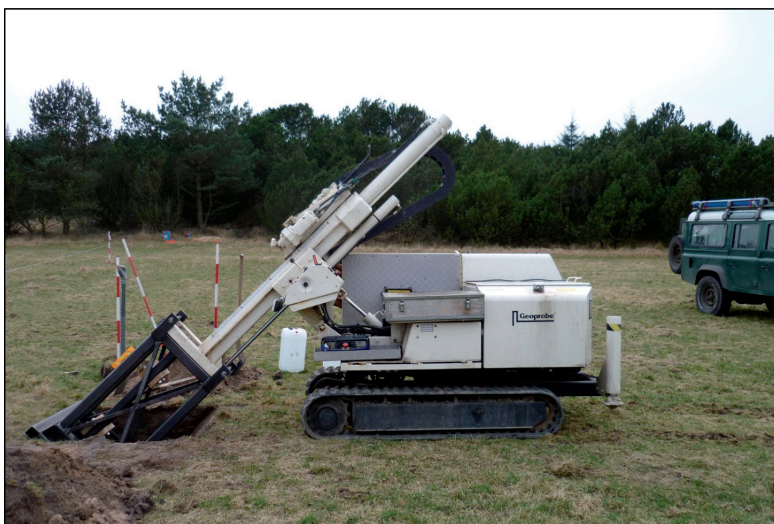
Figure 15. Modified Geoprobe (model 7822DT) drilling main experiment 45 degree inclined CO 2 injection well at Vrøgum field site. Inclined injection wells were employed to enhance dissolution and dispersion of CO 2 into groundwater and limit migration along injection piping.
