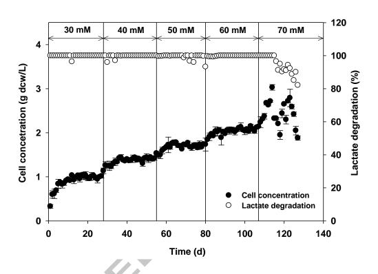
Fig. 3 Daily variation of cell concentration and lactate degradation in the membrane-coupled bioreactor at various operating conditions
