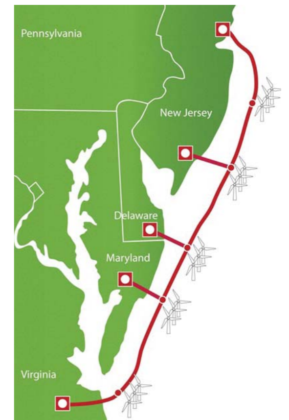
Figure 6. Atlantic Wind Connection project configuration
