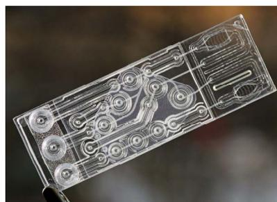
Figure 4: Image of an assembled TOPAS<sup>®</sup> lab-on-a-slide with a dimension of 26 × 76 mm<sup>2</sup>.
