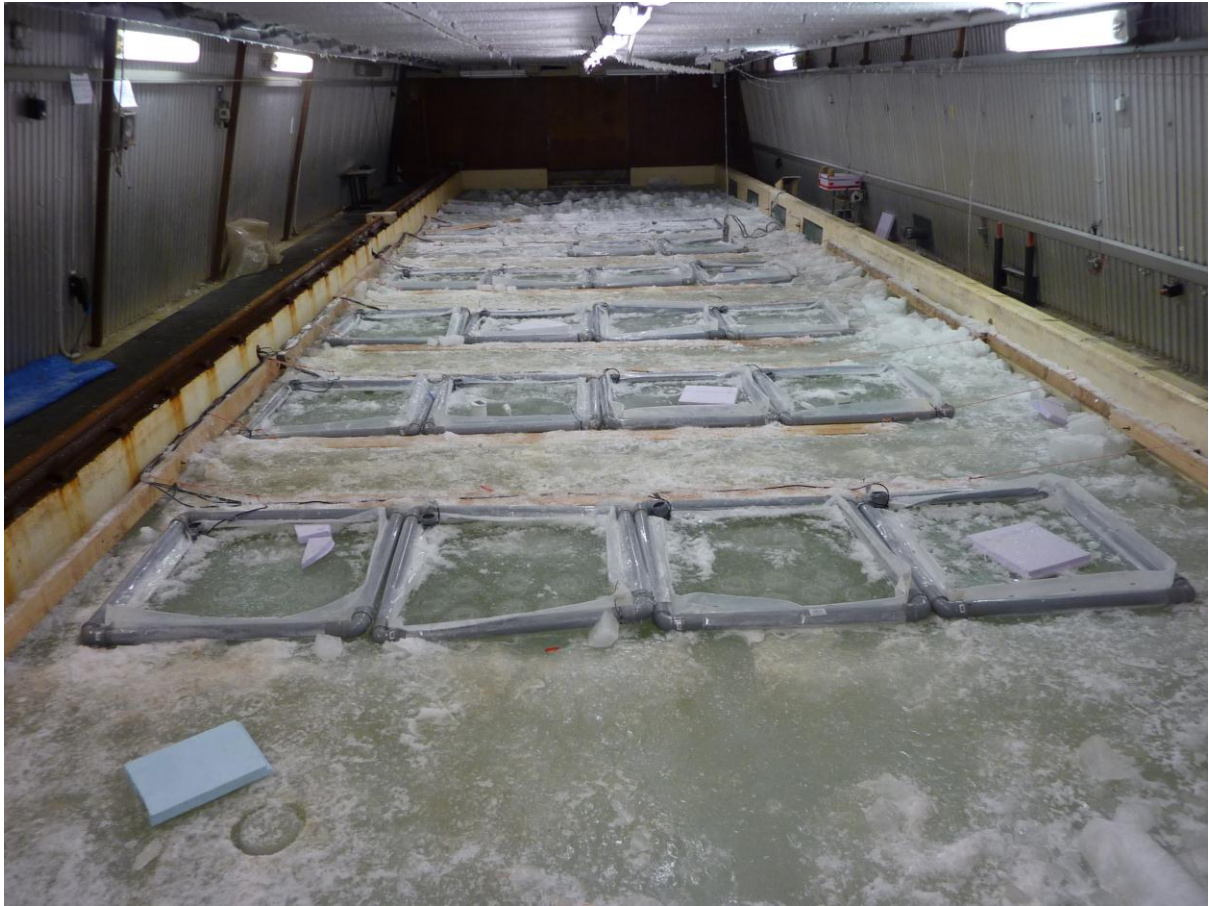
598 Fig. 1: The experimental mesocosms floating in an environmentally controlled ice tank of the 599 Hamburg Ship Model Basin. The foam pads on some of the mesocosms mark the compromised ones 600 after they have been sampled. Note that the lights were on only during sampling (at maximum 2 hours 601 per day) and the rest of the time, the tanks were in darkness.
