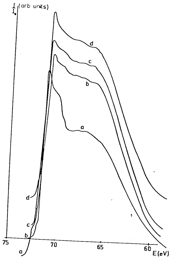
FIGURE 5 The SXES curves: (a) reference (b) alloy measured for 70 min (c) alloy measured for 80 min (d) measured for 120 min.
