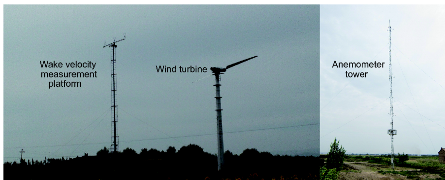
Figure 1 (Color online) Field experiment system, wake-velocity measurement platform, wind turbine, and anemometer tower.
