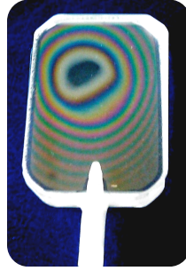
Figure 1.2: Photograph of the nano-cell used for most of the work presented in this thesis, showing the Newton's rings interference pattern. At the centre of the rings, the gap between the windows, and hence the local vapour thickness, is just 30 nm, extending to 2 \mu\text{m} at the bottom of the windows.
