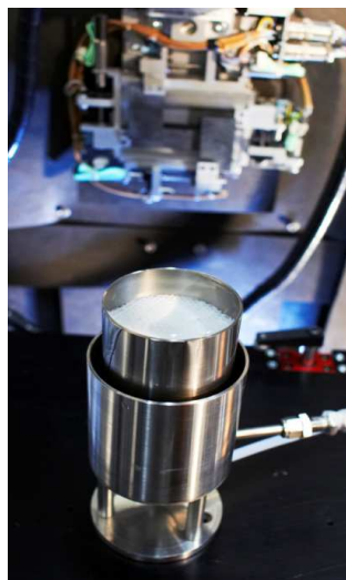
Figure 2.1. Photograph of the overflowing cylinder used in this work in situ on the neutron beamline FIGARO.
