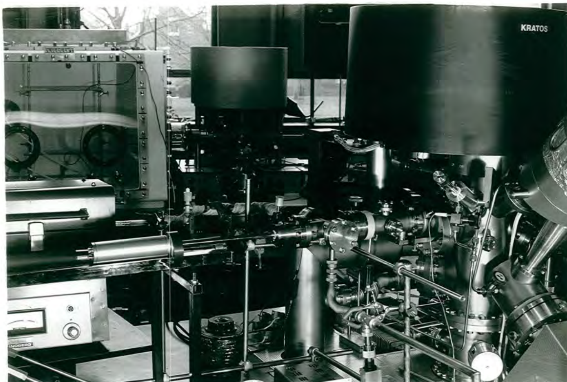
Figure 3.2a. The apparatus shown attached to the insertion lock system of the Kratos ES300 spectrometer.
