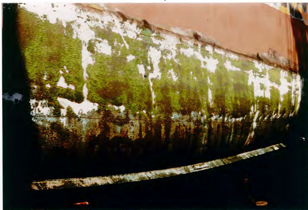
Figure 1.4 Heavily fouled hull showing enteromorpha (green) near water line and ectocarpus lower down
