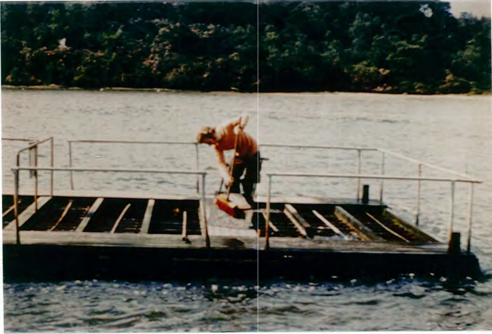
Figure 1.28 B.S.R.A.'s raft for testing new antifouling paints, which is stationed in the estuary at Poole Harbour
