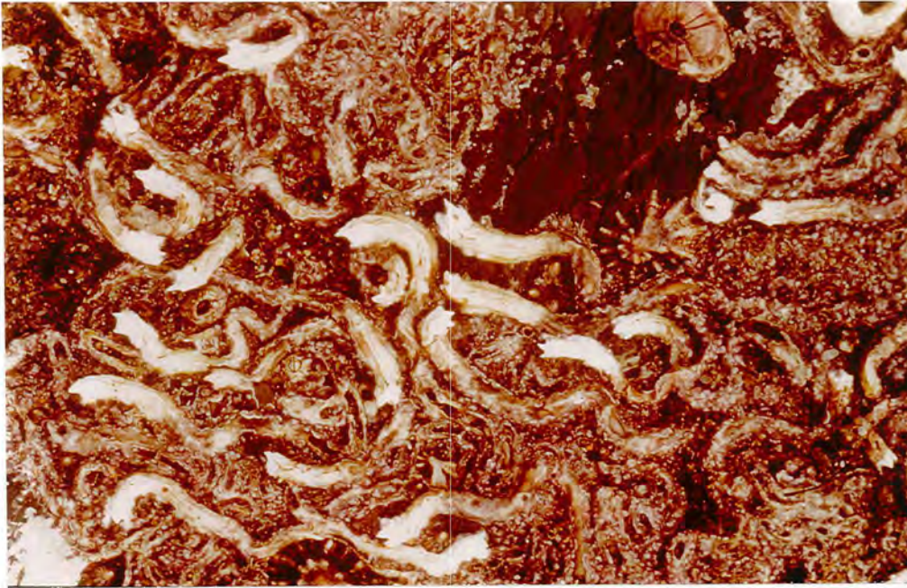
Figure 1.9 Typical calcareous growth resulting from tube-worm fouling
