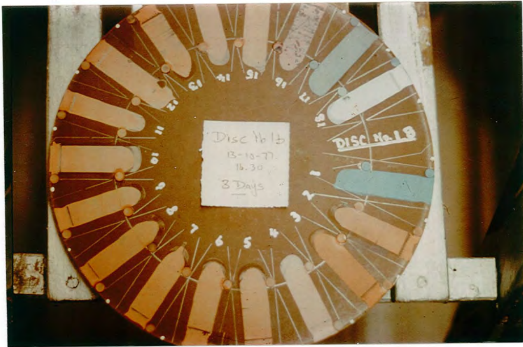
Figure 4.3 A Camrex Disc after sea water Trials
