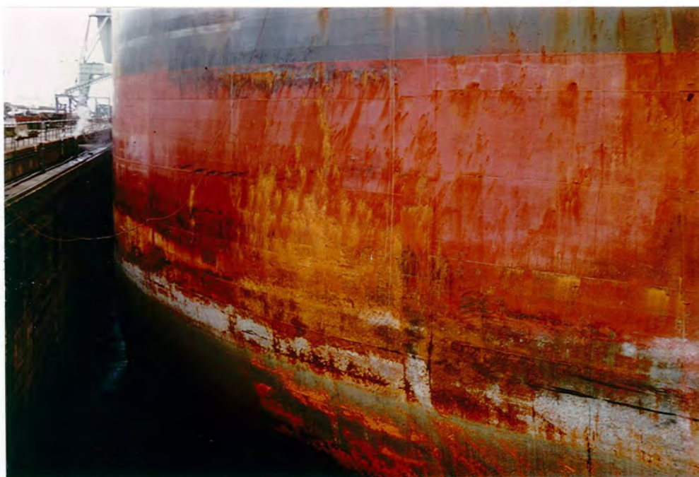
Figure 1.25 Surface Corrosion on the Bows of a Ship
