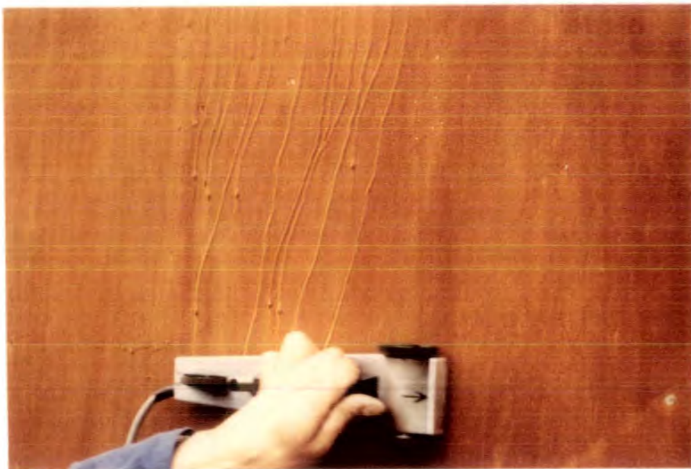
Figure 1.19 B.S.R.A. Roughness Gauge in use
