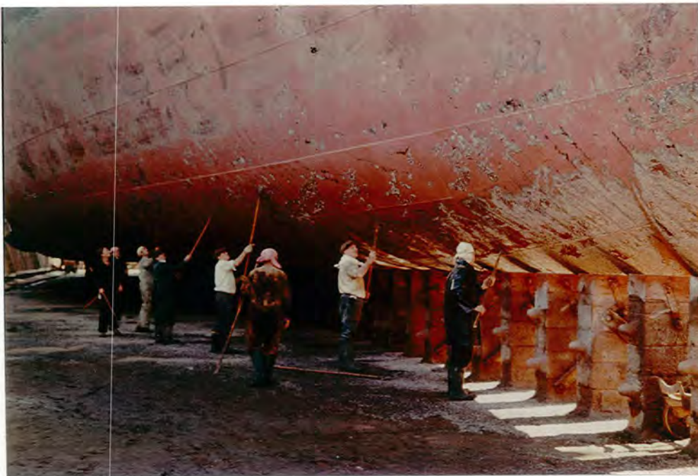
Figure 1.23 Removal of fouling using scrapers
