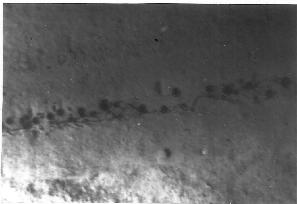
Fig A1.6 : Micrograph of ZnSe:250ppm In after zinc-treatment , showing spherical precipitates decorating a stacking fault. ( X 52000 )
