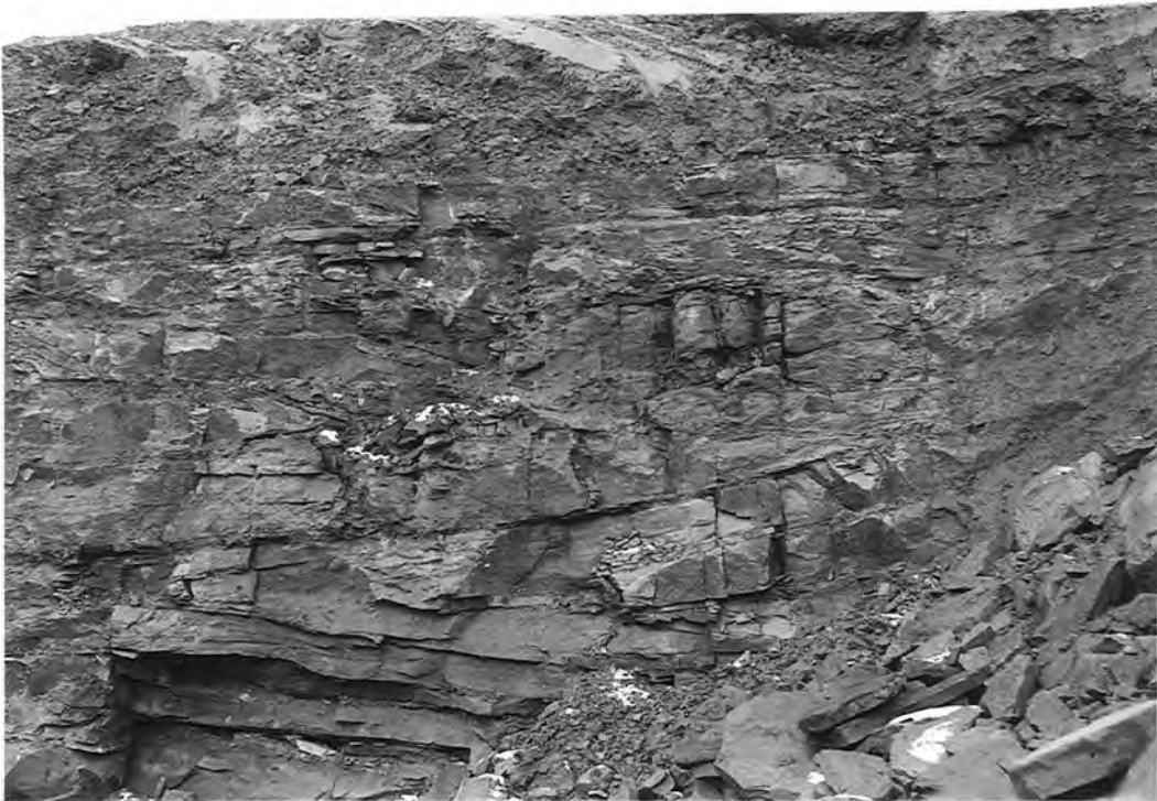
Plate 7.22 - Large trough scours in the upper part of the Fivequarter - 2E00 interval at Edmondsley O.C.C.S. Height of exposure about 6m.
