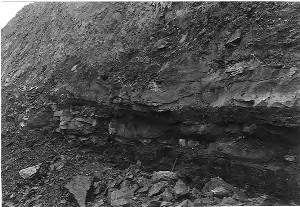
Plate 6.19 - View of the Middle Tilley coal at Rowley O.C.C.S., showing localized, sandstone intra-seam "bands". Hammer is 30cms long.
