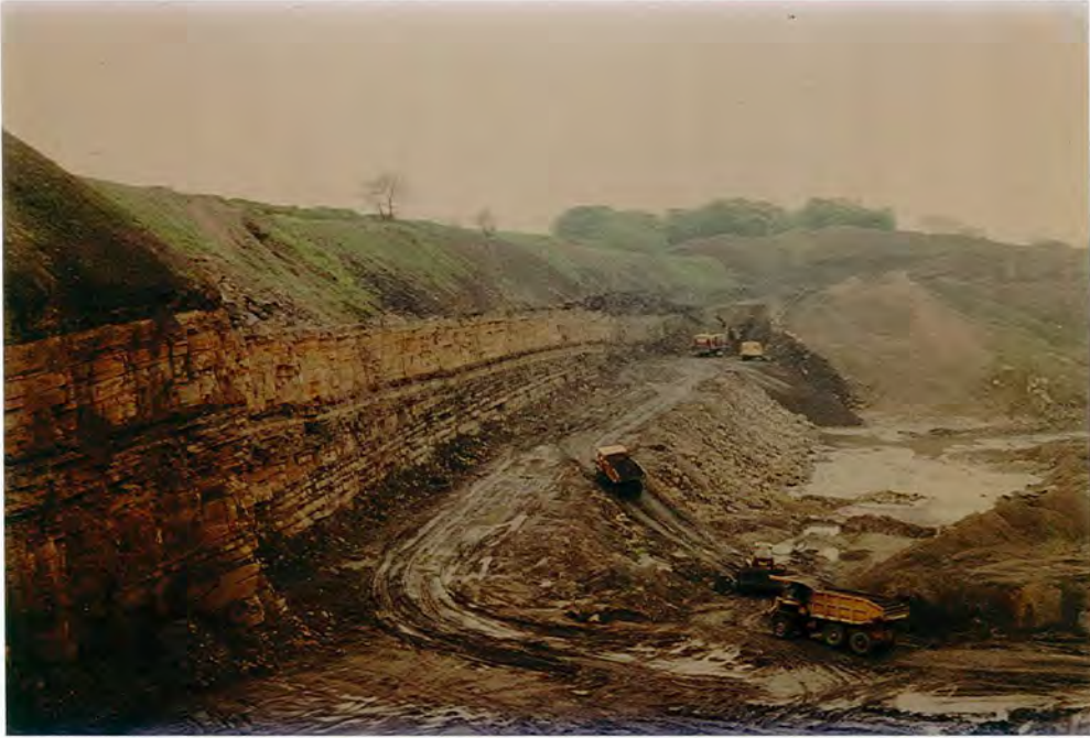
Plate II.5 - Laterally-accreted channel deposit in the Crutchman Sandstone (Lower Westphalian A), exposed at Billinge Hill Quarry, near Up Holland. Height of exposed section about 10m.
