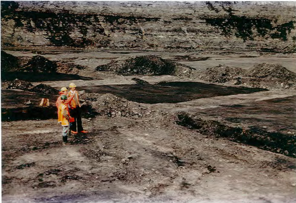
Plate I.4 - "Pillars" of coal left by old mining operations, exhumed during opencasting - Bottom of Broomhill seam, Acklington Extension O.C.C.S.
