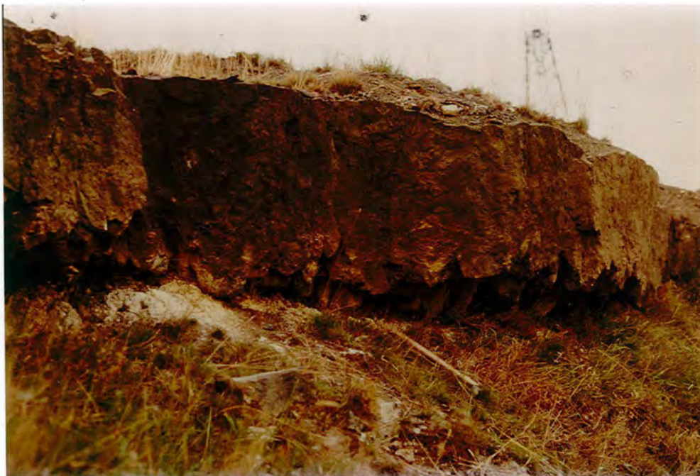
Plate II.2 - The Sheffield Blue Ganister, exposed at Fulshaw Lane, near Langsett. Hammer is 35cms long.
