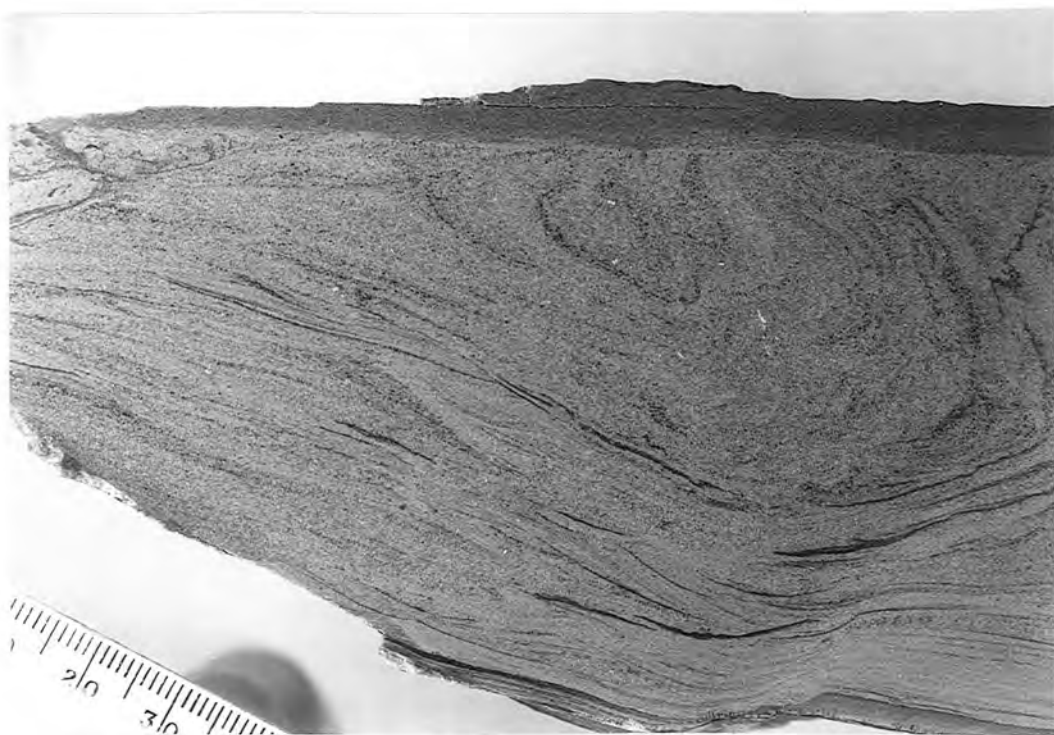
Plate 6.I2 - Load-casted sandstone from the Top Busty - Bottom Tilley interval, Binchester Crags. Scale divisions in mm.
