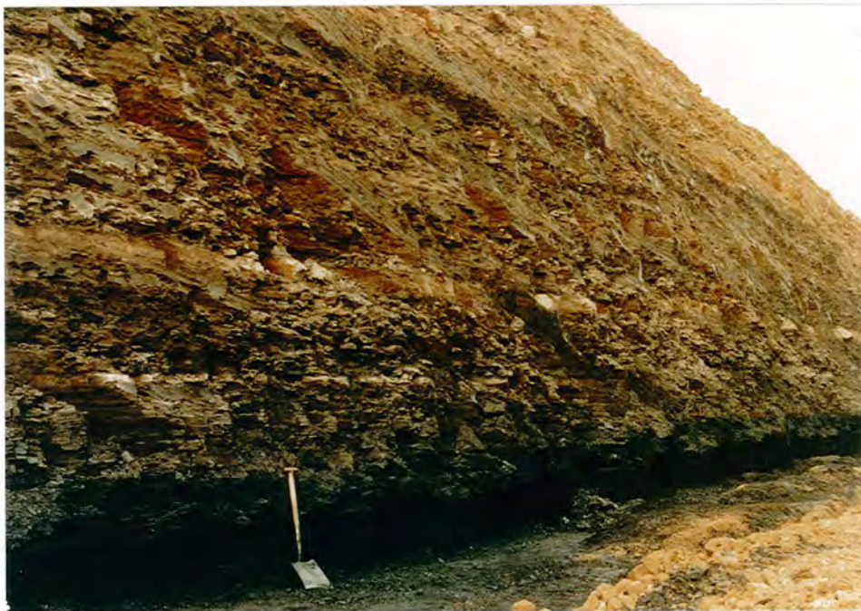
Plate 7.1 - The Hutton coals and overlying sediments at Wooley O.C.C.S. (Cut 3). The sandstone exposed in the upper part of the face is part of the "Low Main Post". Shovel is about 1m high.
