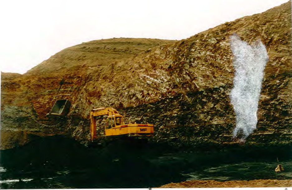
Plate I.3 - View showing removal of coal from an opencast cut - Hutton seam, Wooley O.C.C.S.
