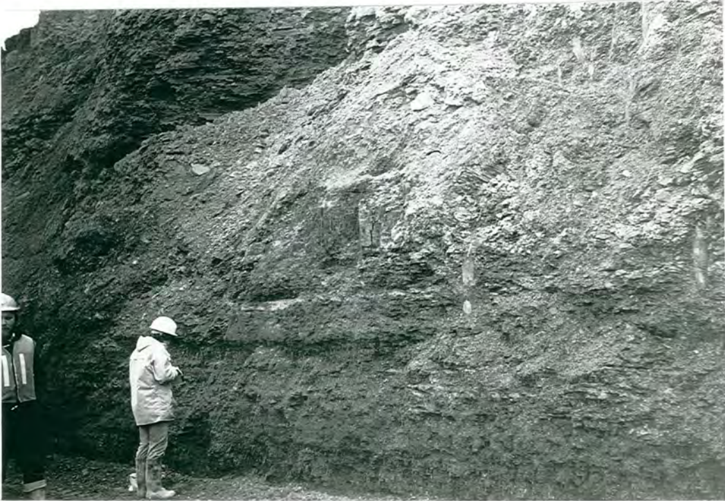
Plate 7.17 - The complex Fivequarter coal at Langley O.C.C.S., showing disturbance by old workings. Geologist is 1.7m high.
