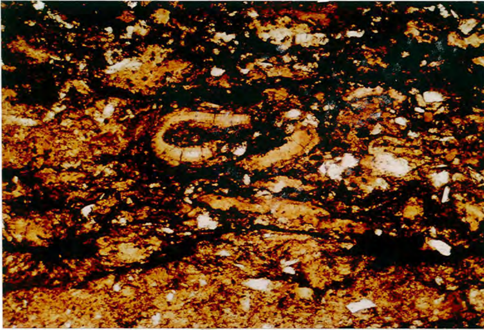
Plate 6.I5 - Vermicular kaolinite crystals in kaolinitic claystone, Middle Tilley coal, Rowley O.C.C.S. Length of photomicrograph 1.2mm. (Plane polarized light).
