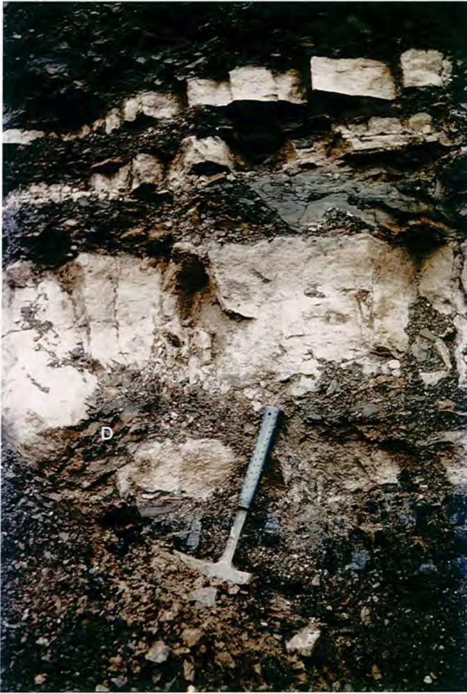
Plate 6.27 - Close-up of Bottom Tilley (PI02) coal and overlying sediments at Buckhead O.C.C.S., showing a claystone dyke (D) which penetrates a sandstone bed and the underlying coal. Hammer is 30cms long.
