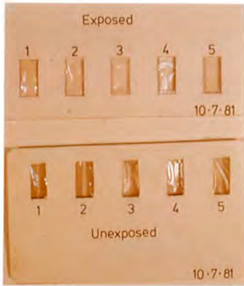
Figure 4.7. Visual deterioration of polymers on exposure to air and light.
