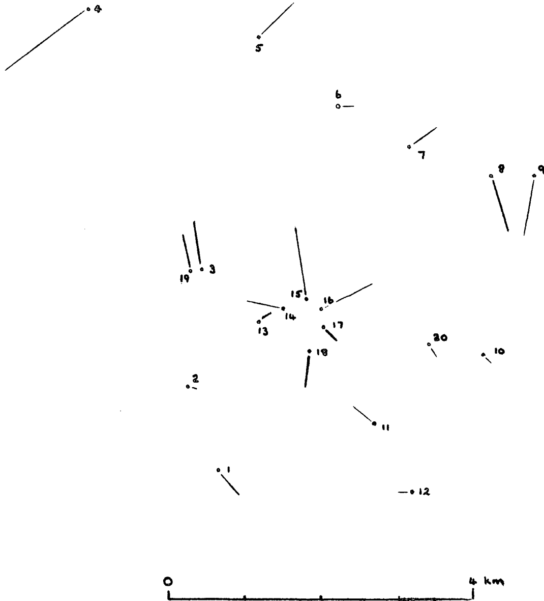
Figure 3.4 Normalised vector differences between the representation of road junction around Darlington at 1:50,000 and 1:250,000 scales
