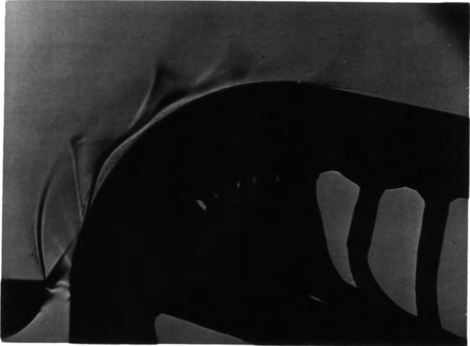
PLATE 10: Shadowgraph, P_a/P_o = 0.267 Slot = 4 mm
