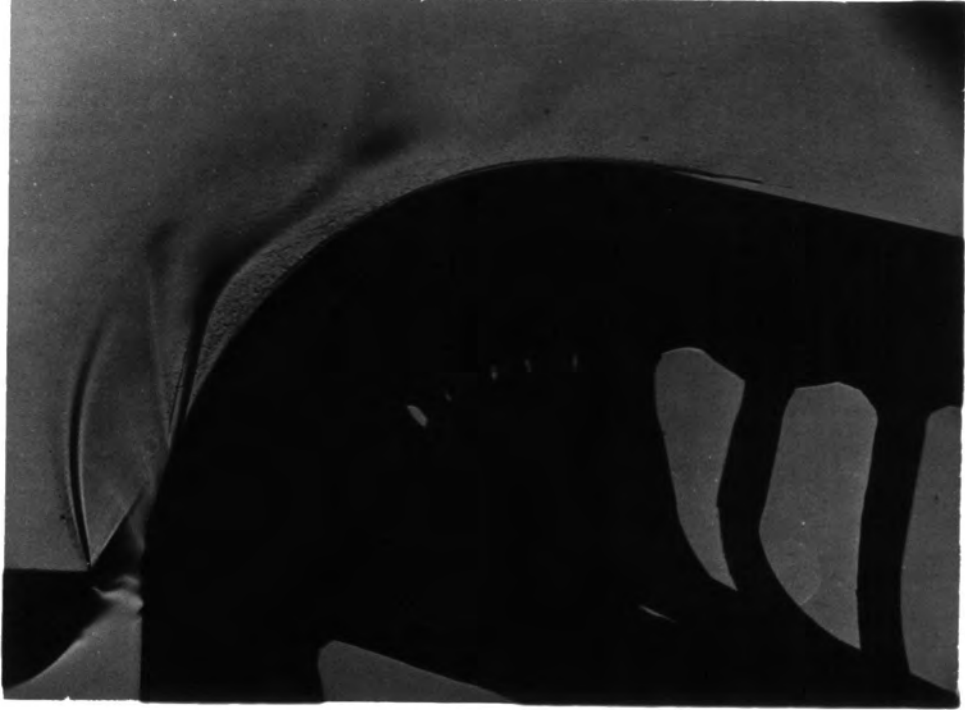
PLATE 11: Shadowgraph, P_a/P_o = 0.241 Slot = 4 mm
