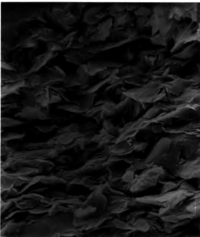
(o) Undisturbed Flockton mudstone (The length is 50 \mu\text{m} ) Preferred orientation in NE-SW direction
