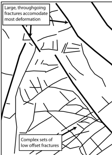
Figure 5.4b. Multiple fracture sets exposed on the wave-cut platform at Praia das Focas show larger, throughgoing NW-SE fractures, with smaller fractures between them. Many of these fractures may be joints, formed either during tectonics or uplift. Identification of offset is impossible, though some of these fractures do show slickenlines.
