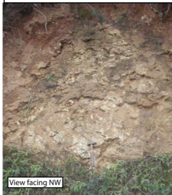
Figure 5.23A. Highly weathered outcrops are found along road sections around Quatis. Fractures often stand out from these, and foliation can sometimes be identified. The quality of the outcrops, however, makes the identification of tectonic features; and distinguishing them from features formed by recent geomorphological processes, very difficult
