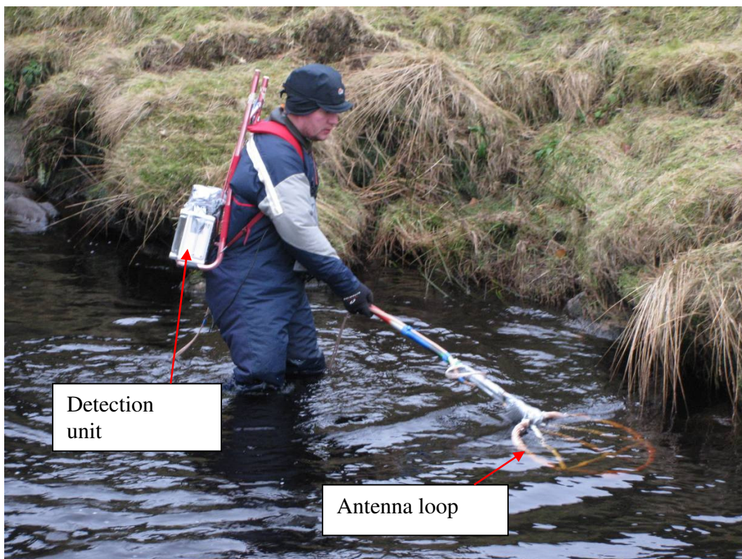
Figure 56: mobile PIT tag detector
