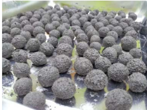
Fig. 1. Pelletized artificial geopolymer aggregate.
