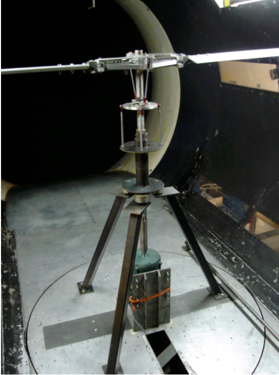
Figure 6: Dynamic Stall rig assembly in the test section of the John J. Harper wind tunnel.
