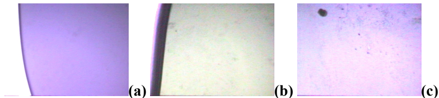
Figure 2. Microscope images (40x) of thick composites of MEH-PPV with different acceptors. (a) 25 \mu m thick composite of MEH-PPV and PDI2. (b) 100 \mu m thick composite of MEH-PPV and PDI2. (c) 25 \mu m thick composite of MEH-PPV and PCBM- C_{60} .
