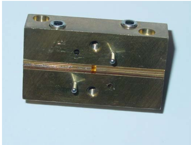
Fig. 11. Photo of the assembled Silicon waveguide block.
