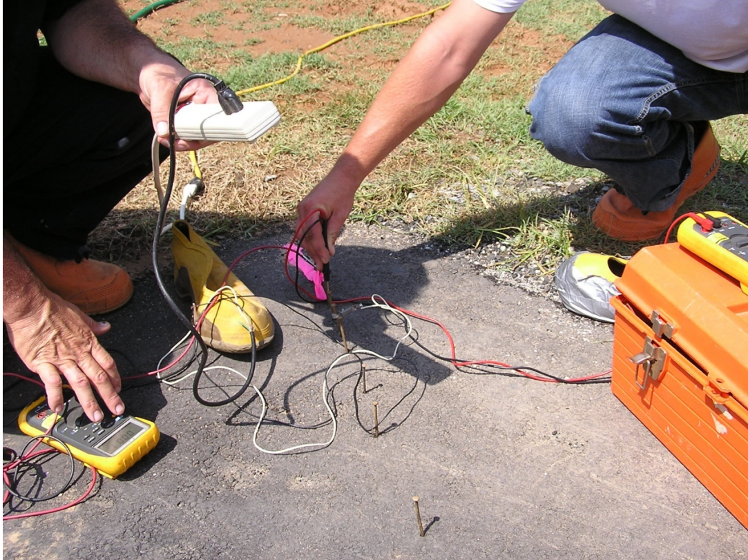
Figure 2-7: Four-Pin Measurement of Asphalt Resistivity using Nail Electrodes
