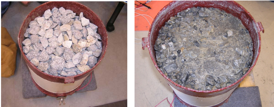
Figure 2-8: Gravel Resistivity Measurements Using Cylindrical Test Device (#34 Washed Gravel on the left and 1½" Crusher Run Gravel on the right)
