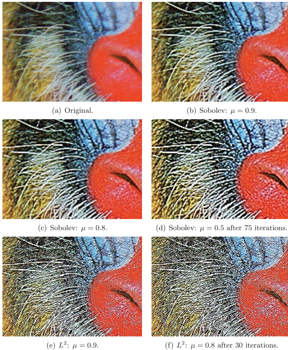
Figure 5. Stable Sobolev sharpening vs. unstable L^2 sharpening. (b), (c) For \mu = 0.9, 0.8 the discretized gradient descent PDE (5.6) converges to a local minimum (though the true continuous PDE would not). (d) For \mu = 0.5 the PDE does not converge but does yield a family of sequentially sharper images. In (e) and (f), we see that the L^2 gradient descent PDE very quickly exhibits instabilities and oscillatory behavior (diffusion was performed on the luminance component only).
