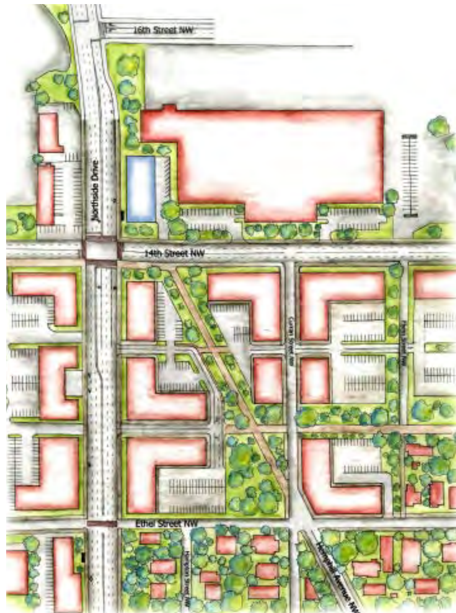
Figure 18. Illustration of the ultimate recommendation, that is, to convert that part of Hemphill between 14th and Ethel Streets into a cycle track street, eliminating its intersection conflict with 14th Street
