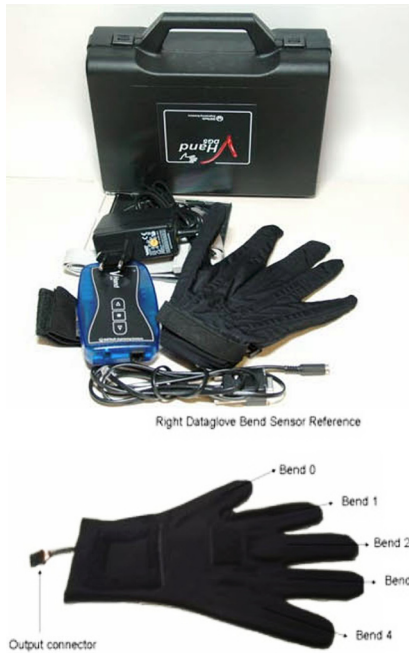
Figure 1. Two images of the DGTech VHand glove. The picture above shows the complete DGTech glove package including the serial link, com port, and power adapter.
