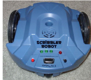
Figure 3. The Scribbler robot used to test the teleoperative capabilities of the VHand glove. The Scribbler's API has built-in functions to control the movement of the robot, play sound bytes, and activate the onboard LEDs.
