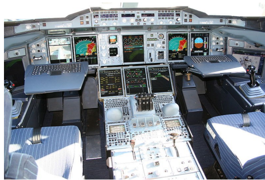
Figure 39: Airbus A380 Cockpit (copied from [43])
