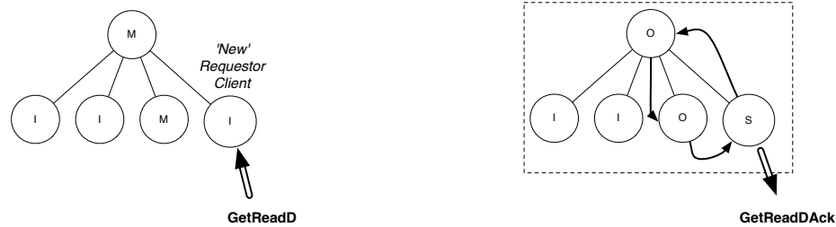
Figure 31 - Local GetReadD Get sequence (Request and Response) in a MOSI protocol that currently holds write permissions.
