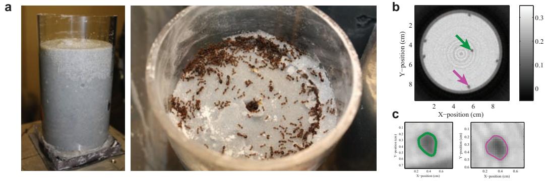
Figure 8.1: Overview of the X-Ray CT digging trials. a) Digging arena consisted of a circular plastic, or aluminum container of diameters 8.2 or 3.8 cm, filled to a height of approximately 12-15 cm with a simulated soil of monodisperse 50, 210, or 810 \mu\text{m} diameter, wetted, glass beads. b) A horizontal cross-section from X-Ray CT reconstruction at a depth of 6.8 cm from the surface. Top and bottom arrow indicate two tunnels not adjacent to arena wall. Four other tunnels are present but against the tunnel wall. c) Cross-section of the top (left) and bottom (right) tunnels from (b) with extracted tunnel shape from active contours method shown as green (left) and purple (right) lines.
