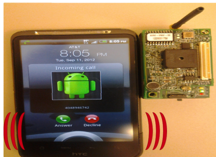
Figure 9: Incoming Call Experiment (Left: Android device; Right: MTS310CB with accelerometers)
