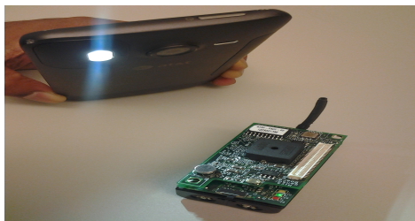
Figure 6: Morse Code Experiment (Left: Android device; Right: MTS310CB with light sensors)
