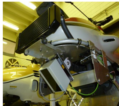
Figure 9. The second RMAX with nose-mounted laser range finder.
