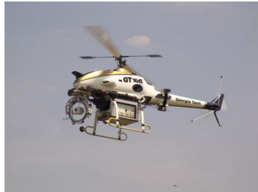
Figure 8. Yamaha RMAX instrumented with Differential GPS, inertial measurement, magnetometer, sonar altimeter, and camera.
