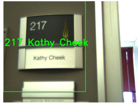
Fig. 5. This sign is recognized and a measurement is made in the mapper. GoogleGoggles has read both the room number and the text, so this sign can be used for data association.
