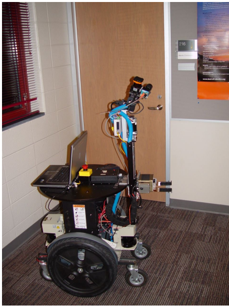
Fig. 4. The Segway RMP 200 with LMS 291 laser scanner for wall measurements and a Prosilica 650c camera with a Hokuyo UTM30 laser scanner on a PTU-46-70 pan-tilt unit. Four caster wheels were added for stability. The robot is shown in a position typical of reading a door sign.
