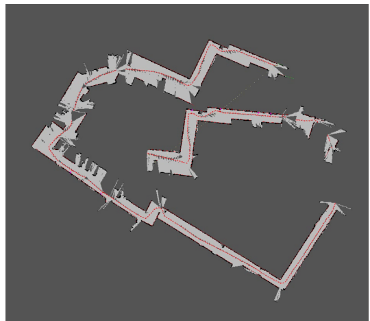
Fig. 11. The robot has completed the long loop around the building, but has not yet found a sign match to perform a loop closure. Note that there is significant error in this map when the door signs have not been re-observed.
