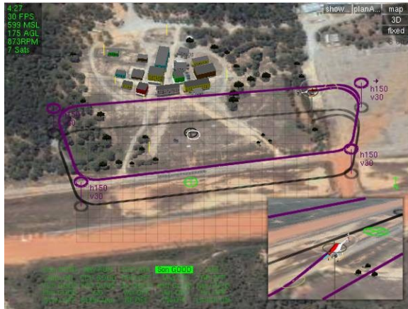
Figure 10: 3D view of ground path for first test of single scan algorithm (South up).
