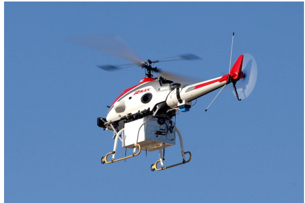
Figure 4. Yamaha RMAX based research UAV utilized for this effort, 10.2 ft main rotor
