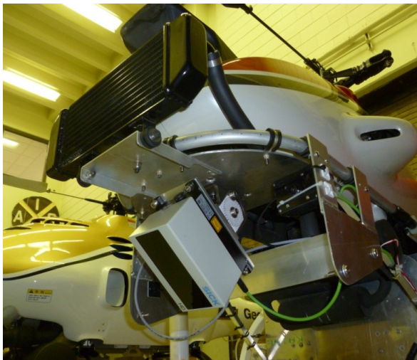
Figure 5. Sick LD-MRS Laser scanner mounted under the nose of the aircraft, able to see down and forward (sensor rotated 90 degrees in roll, 40 degrees nose down pitch)
