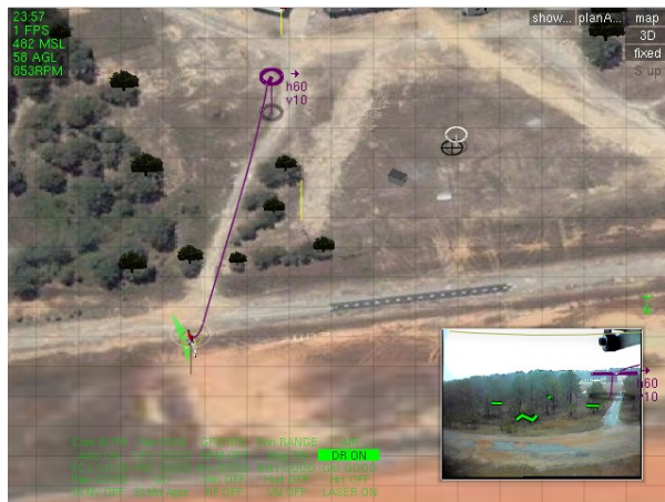
Figure 19. Ground station view of the "down-the-road" mission. Main window is generated from a combination of ground station data and static aerial photography. The sub-window is on-board video with ground station data overlaid.
