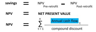
Figure 46: Net Present Value calculation for a facade retrofit
