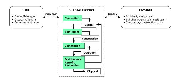
Figure 3: Building product lifecycle phases and decision stages including retrofit decision (constructed based on (Straube et al. 2005)
