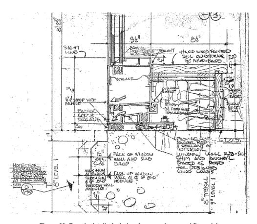
Figure 23: Facade detail of window frame and exposed floor slab
