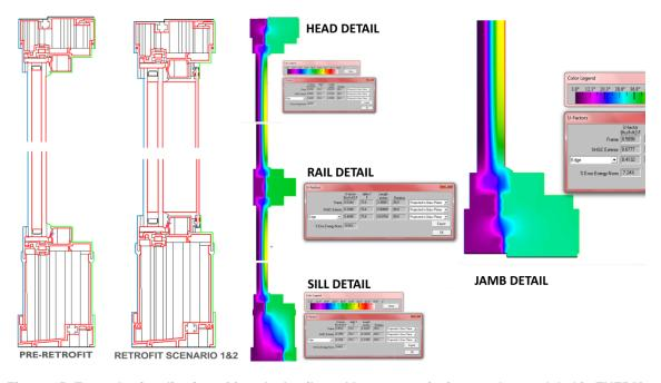
Figure 45: Example visualization of façade details and heat transmission results, modeled in THERM
