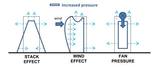
Figure 21: Classification of air pressure causing air leakage in the façade
