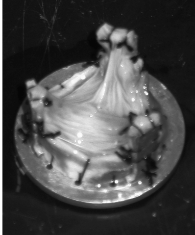
Figure 4-7. The native tissue valve model of the normal aortic valve, trimmed and sutured to a tri-stented ring.
