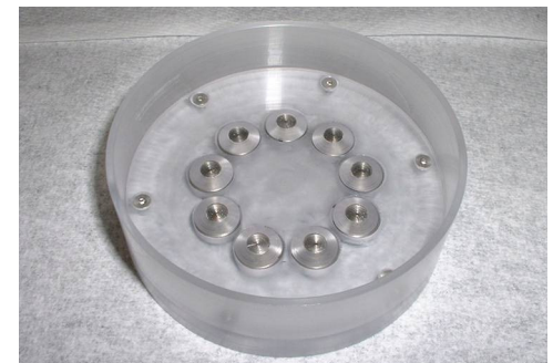
Figure I.5: Plate, agarose bed and cover assembly.
