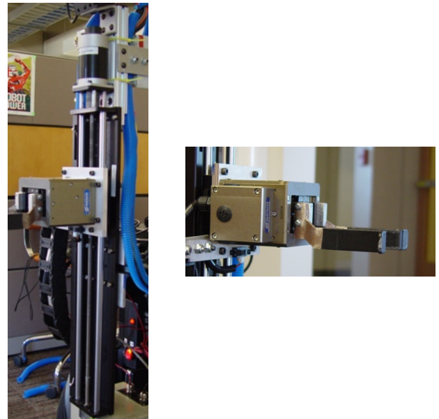
Fig. 2: Manipulator and gripper used on the Jeeves platform.
