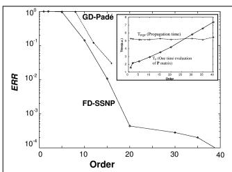
**Figure 1** Propagation error (ERR) as a function of the order of approximation for the derivative (Eq. 7) for the graded-index waveguide [3] tilted at  $50^{\circ}$ . For the FD-SSNP method, N=900, and step size  $0.05~\mu m$ .
