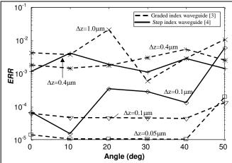
**Figure 2** ERR as a function of waveguide tilt angle. The order used for graded-index waveguide is 35 and for the step-index waveguide is 30.
