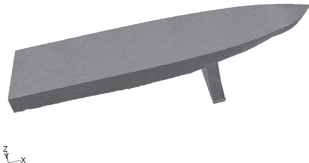
Fig.8.2 The Cartesian coordinate system o-xyz and mesh for a ship hull
