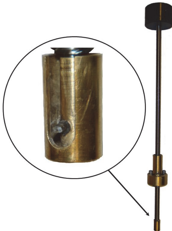
Figure 5.6 10mm helical rib cutter with ball nut and cutting bucket.
