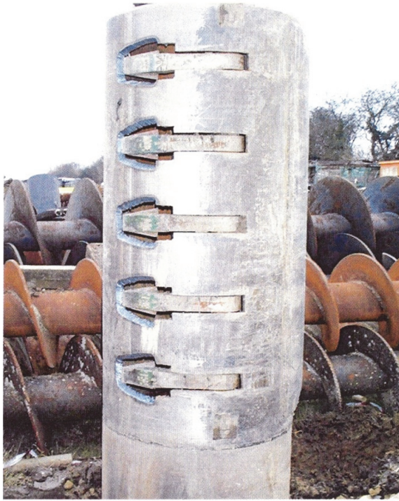
Figure 2.12 Expanded Piling construction issue rib cutting tool.
