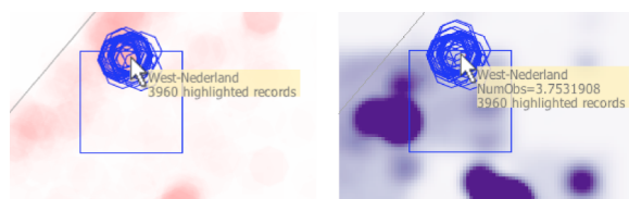
Figure 1: Observation footprint map (left; blue footprint outlines) and density estimation map (right), indicating the extents and numbers of observations at the mouse cursor.
