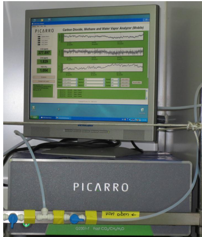
Fig. 4.1.4: CO 2 , CH 4 , H 2 O gas analyser “Picarro G2301-f” installed onboard RV ALKOR.
