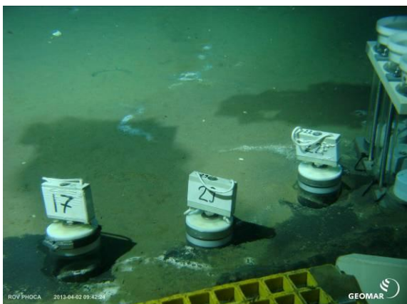
Fig. 4.2.3c: Pushcore sampling of bacterial mats at the Hugin fracture.
