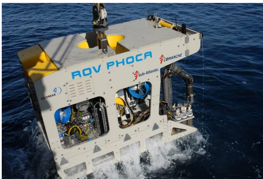
Fig. 4.2.2: ROV PHOCA during recovery; carrying a six-pack with push cores on its porch.
