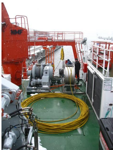
Fig. 4.2.1: Deck-setup of cabling, capstan winch and laid out tether cable on upper deck of RV ALKOR (Photo: ROV Team GEOMAR)
